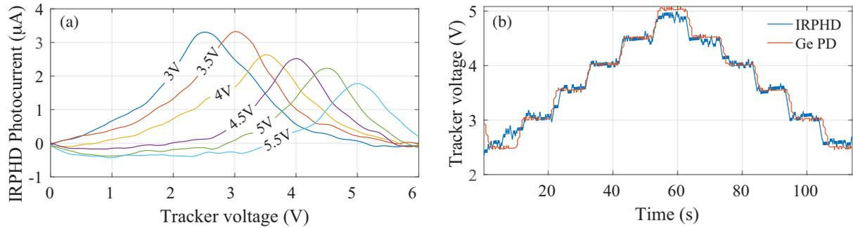
Fig. 2: (a) The IRPHD photocurrent as a function of the tracking ring voltage at various sensing ring voltages (indicated as legends on the line plots). (b) Tracker voltage to maximize the photocurrent (from the IRPHD and Ge PD) at various sensing ring voltage setpoints across time, implemented using a maximum search algorithm (the dither signal can be seen).
