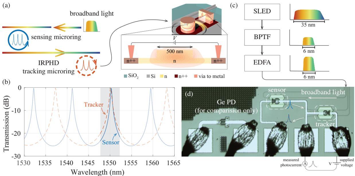
Fig. 1: (a) Layout of the photonic sensor consisting of two microrings, a sensor and a tracker, using a broadband source. (b) Frequency spectrum of each microring across the spectrum of the SLED shown in (c). The shaded region shows the resonance of each ring over a bandwidth of 6 nm, as filtered by the BPTF in (c). (c) Block diagram of our experimental setup. (d) Optical microscope image of a test device.
